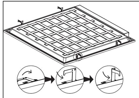
**3.** Insert luminaire into T-bar ceiling grid. Secure safety cable to connection hole as needed to meet local seismic requirements. Safety cable and method of attachment to the building provided by contractor according to local building codes.
