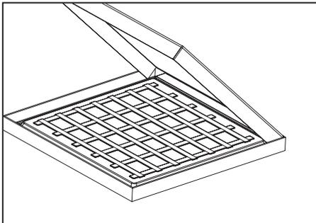
**2.** Lift up four mounting clips on the sides of the luminaire. You can do it by hand (Do wear work gloves) or use pliers.
