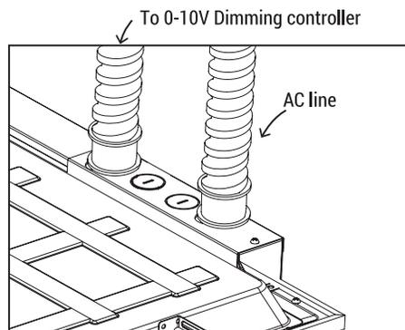
**6.** Follow wire connection instructions. When using the 0-10V dimming controller Run wires from controller through a different knockout than the AC input wire. Don't forget to return the electrical enclosure cover and tighten the screws.
