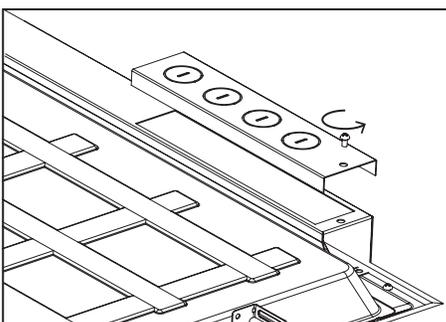
**5.** Plug in AC line (L and N, and GND) to the LED Driver using 18-14AWG Wire. When connecting 0-10V dimming controller, wires must run through a separate knockout hole equipped with an appropriate electrical fitting.
