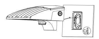
Connect the corresponding terminals according to the wiring diagram, connect L, N, and ground wires properly. (Fig 4)
