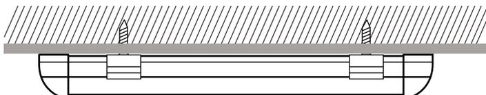
1. Gently press the tube into the metal clips until it is secured properly.
