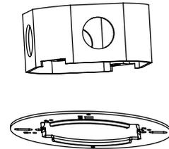
4. Attach the bracket to the junction box. Using mounting screws.
