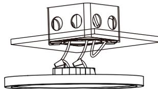
6. Place the fixture and make sure the springs are squeezed and snapped into the bracket.
