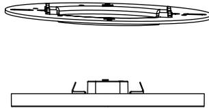
3. Match the hole position on the bracket to the J-Box.
