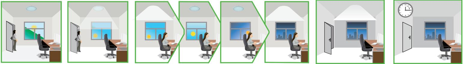
The lamp will not switch on when natural light is sufficient, even there is motion detected.
