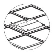
**3**. Lay fixture into T-grid.
