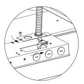
**6**. Make sure all electrical connections are properly connected. Attach the wiring access cover plate.
