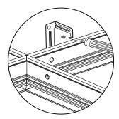
**4**. Bend tabs flush against T-grid in order to clear corner for ceiling tile.
