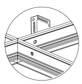
**7**. Bend out mounting tab 90° on each corner of the fixture.
