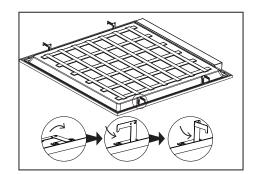
Insert luminaire into T-bar ceiling grid. Secure safety cable to connection hole as needed to meet local seismic requirements. Safety cable and method of attachment to the building provided by contractor according to local building codes.
