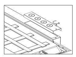
Plug in AC line(L and N, and GND) to the LED Driver using 18-14AWG Wire. When connecting 0-10Vdimming controller, wires must run through a separate knockout hole equipped with an appropriate electrical fitting.
