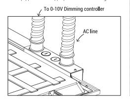
Follow wire connection instructions. When using the 0-10V dimming controller Run wires from controller through a different knockout than the AC input wire. Don't forget to return the electrical enclosure cover and tighten the screws.
