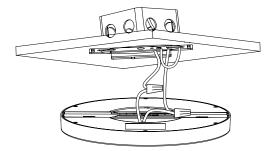
**6** After installing the mounting bracket, push the product in the direction of the mounting bracket hole position.
