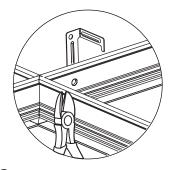
**2**. Use side cutters tools to adjust each tab to height of T-grid.
