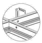
**1**. Bend out mounting tab 90° on each corner of the fixture.
