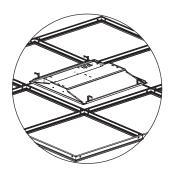
**3**. Lay fixture into T-grid.
