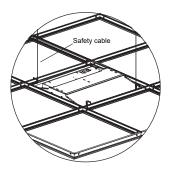
**5**. Use a #8×1/4" sheet metal screw to fasten fixture to T-grid. Use a hanger wire to tie off appropriately in accordance with local building codes (screws and hanger wires not provided).
