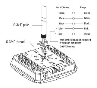
2. Rotating the pole to make it secured with fixture.
