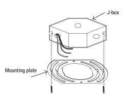
Connect supply wires to wires on fixture with wire nuts or push wires into Quick Connector. Connect white to white, black to black, and copper wire to copper wire as grounding connection.
