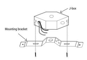
Connect supply wires to wires on fixture with wire nuts or push wires into Quick Connector. Connect white to white, black to black, and copper wire to copper wire as grounding connection.
