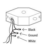
Completing the installation by attaching the fixture into the mounting plate tightly to the j-box. Attach the diffuser by twisting and lock the diffuser in place.
