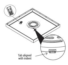
5. Using sticker on the fixture (reference point for mounting tab) and on the ceiling as reference point, lift fixture up to the ceiling and rotate clockwise until fixture is secured (45-degree turn until it locks).
