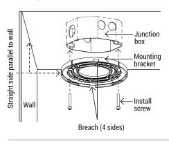
Before working wire connections, attach to hook side of safety cable on mounting bracket.
