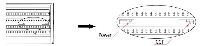
The DIP switches of the CCT from left to right are 5000K, 4000K and 3500K. Power Dip switch From left to right: highest power, middle power, lowest power. Remove the pc diffuser cover and backplane before switching.
