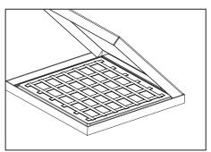
Lift up four mounting clips on the sides of the luminaire. You can do it by hand (Do wear work gloves) or use pliers.
