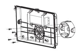
**METHOD 2**: Drill holes at the required three mounting points, mount the fixture by securing mounting screws (not provided) through the drilled holes, and seal the screw heads with appropriate waterproofing material.
