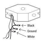
**5.** Arrange the wires into the Junction Box. Align appropriate slots in the disk light with the holes in the Junction Box. Use 2 screws to attach the disk light, flush with the ceiling.
