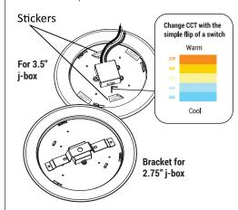
Connect the supply wires to the wires of disk light by using 3 wire nuts. Attach white to white, black to black, green to the ground wire.
