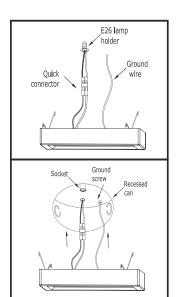
Insert wires into Quick connector. Black to black and white to white. Attach ground wire to ground screw in recessed can.
