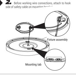
4. Attach provided to indents (opening) of the Mounting Bracket and align mounting tabs on back of the fixture with indents in the Mounting Bracket.
