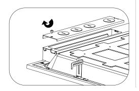
Lift up four mounting clips on the sides of the luminaire. You can do it by hand (Do wear work gloves) or use pliers.
