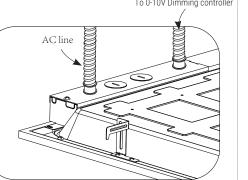
**6** Follow wire connection instructions. When using the 0-10V dimming controller Run wires from controller through a different knockout than the AC input wire. Don t forget to return the electrical enclosure cover and tighten the screws.
