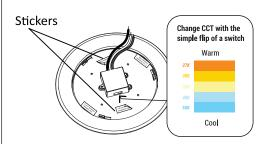
Connect the supply wires to the wires of disk light by using 3 wire nuts. Attach white to white, black to black, green to the ground wire.
