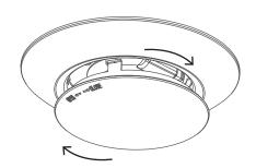
Remove the two stickers at the disk light back that read as 2.75" / 3.5" Junction Box installation hole to reveal the screws lots. The bracket use for 2.75" Junction box. Select lamp color desired with the CCT switch.
