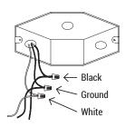
Arrange the wires into the Junction Box. Align appropriate slots in the disk light with the holes in the Junction Box. Use 2 screws to attach the disk light, flush with the ceiling.
