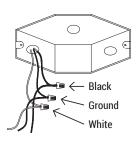
Arrange the wires into the Junction Box. Align appropriate slots in the disk light with the holes in the Junction Box. Use 2 screws to attach the disk light, flush with the ceiling.
