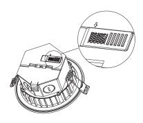
**6)** Connect the hardwire pigtail to the main power line. Black goes to black and white to white. Use the wire nuts provided to ensure there is a secured connection .
