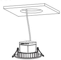
**9)** Pull the spring clips on the slim microdisk up and gently guide through the ceiling hole until the clips snap.
