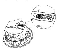
**5)** Install the E26 adapter into the CAN socket
