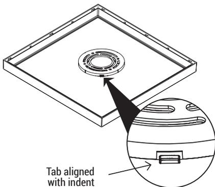
5. Using sticker on the fixture (reference point for mounting tab) and on the ceiling as reference point, lift fixture up to the ceiling and rotate clockwise until fixture is secured (45-degree turn until it locks).
