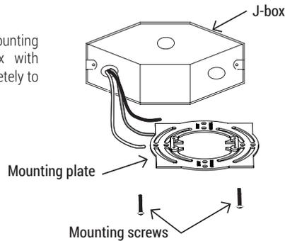
2. Connect supply wires to wires on fixture with wire nuts or push wires into Quick Connector. Connect white to white, black to black, and copper wire to copper wire as grounding connection.
