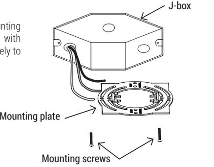
**2.** Connect supply wires to wires on fixture with wire nuts or push wires into Quick Connector. Connect white to white, black to black, and copper wire to copper wire as grounding connection.
