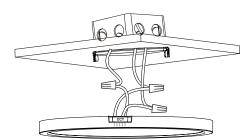
• After installing the mounting bracket, push the product in the direction of the mounting bracket hole position.
