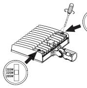
**Step 1:** Open the metal plug and plastic plug counterclockwise with a screwdriver, then slide the switch up and down to adjust the power controller, CCT controller or photocell controller in your demand.
