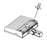
**Step 2:** After adjusting the required control function, tighten the metal plug and the plastic plug clockwise.
