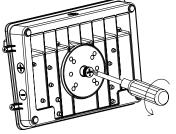
Use a screwdriver to remove the plug, Attach the EVA cotton pad to bottom.
