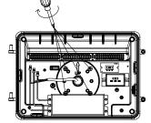
Lock the bottom shell on the mounting seat with screws,Connect the L, N and G wires to the power supply.
