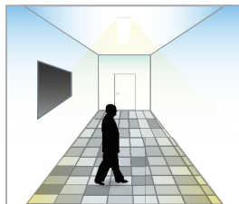
With insufficient daylight, the sensor turns light ON when motion gets detected.
