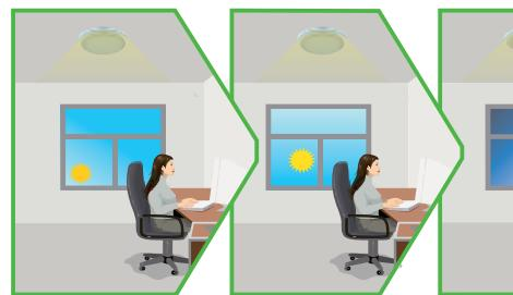
The light turns on at full or dims to maintain the lux level. The light output regulates according to the level of natural light available.
