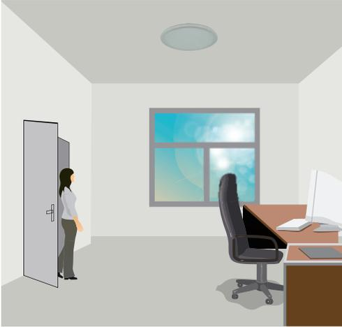
With enough ambient brightness, sensor will keep the light OFF even though it detects heat.
