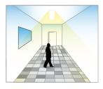
When the natural light is sufficient or dark, movement is detected and the light will turn on 100% brightness.
