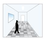
With sufficient daylight, the sensor keeps light OFF even motion gets detected.
