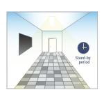
After holdtime, sensor dims light to standby dimming level for standby period. If the standby period has been set as Os, sensor turns light OFF automatically after holdtime.
