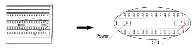
The DIP switches of the CCT from left to right are 5000K, 4000K and 3500K. Power Dip switch From left to right: highest power, middle power, lowest power. Remove the pc diffuser cover and backplane before switching.
